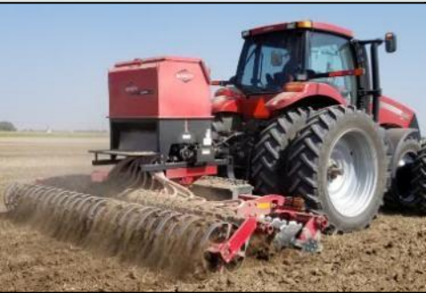
Broadcast Incorporation- BI: Gandy Air Seeder; Horsch Joker, Degelman Pro Till, Vertical Tillage Tool (no row spacing)
